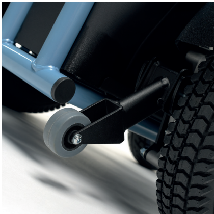
Anti-tipping and taxi hooks for additional safety
